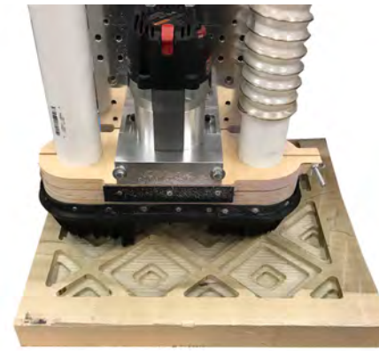
CNC machine carving the wood tile
