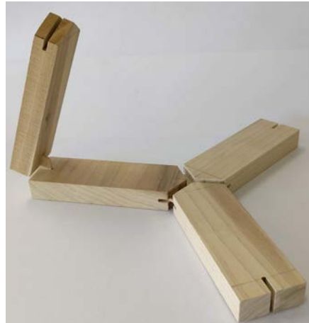
- Connection study with a triangular joint
