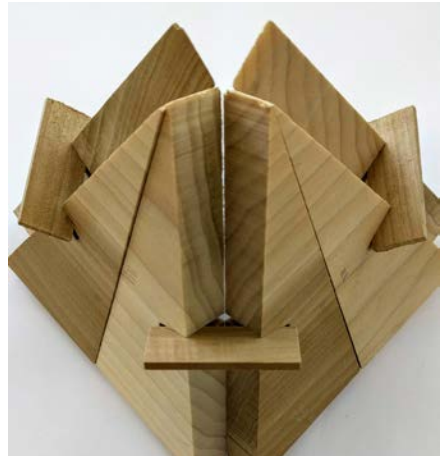
- Connecting using spline joint
